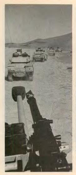
S.A armored cars on patrol. Browning .30 cal. light machine guns and 90mm main guns are kept covered until put into action.
